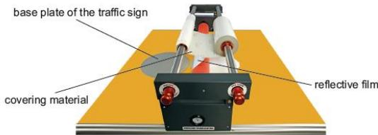
If it is necessary to apply two pieces of prismatic sheeting side by side (splicing), they must not overlap. Depending on the format, the gap should be approximately 1 mm [0.04 inches]. Please ensure a right side of the film web is always bonded to a left side, thus ensuring the uniform orientation of the film's honeycomb structure (shown below).
