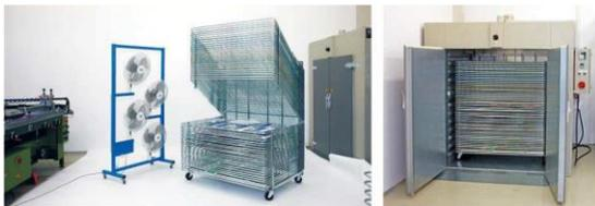
Drying conditions can be further optimized by using convection ovens. These closed systems permit a low-dust drying phase at constant temperature, low air humidity and do not subject the operator to solvent vapors.
